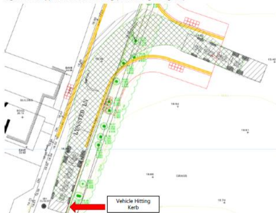
Figure 5: Unsupported Vehicle Tracking (Left Turn Egressing Site)
