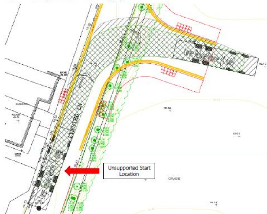
Figure 4: Unsupported Vehicle Tracking (Right Turn into Site)
